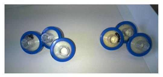
Figure 9: The Convergence MFI/SDI 0.45 micron filters used to derive the MFI/SDI of the ASRRO feed water (left) and the BWRO feed water (right) (date: June 19, 2015).
