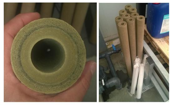
Figure 10: Pre-filters (1 micron, red-brown-coloured) of 'RO' on June 24, 2013. The white filters indicate the colour of unused pre-filters.
